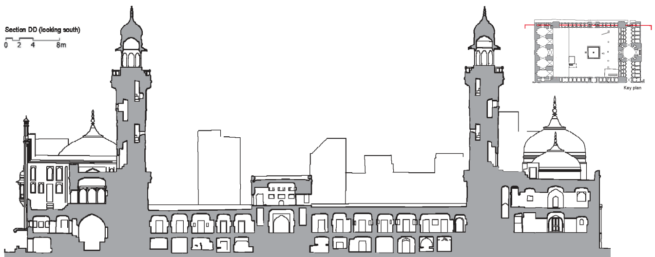
Figure 20: Longitudinal section of the mosque through the northern most section of minars, hujras, shops at level 0 and main prayer chamber
